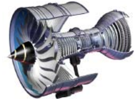
Sixty years of technology development: Left – A cutaway General Electric J31 (I-16) turbojet engine based on Frank Whittle's W.1/W.2B (1940s). Right – Rolls-Royce Trent 1000 (2000s).
