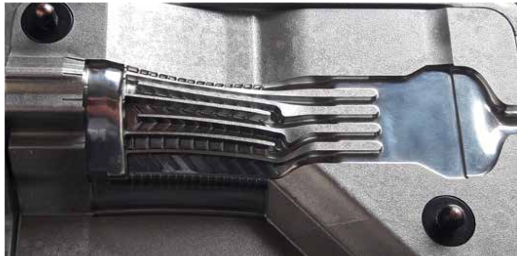
Gardner Blade's NATEP project researched how additive manufacturing could improve the control of cooling in die blocks
